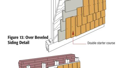
1 x 3 or 1 x 4 nailing strips spaced according to exposure of Certi-label Western Cedar shingles or shakes, regardless of single or double course. (See pages 6-7)
