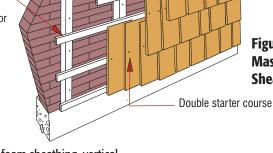
Figure 14: Over **Masonry or Foam Sheathing Detail**
