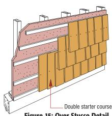
Figure 15: Over Stucco Detail
