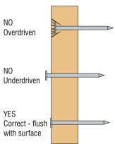
Figure 4: Nail Driving Detail
